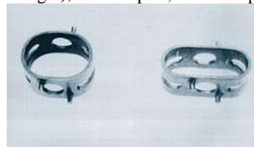
**Fig 7.** Spinal vertebrae spacer shown in the martensitic state (left) and deployed superelastic state (right)
